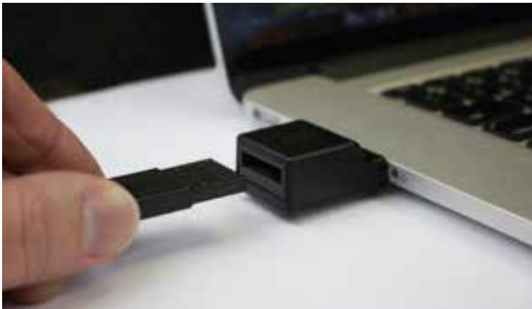
Figure 2: An adapter is used to allow a non-standard memory device to plug into a standard USB port
